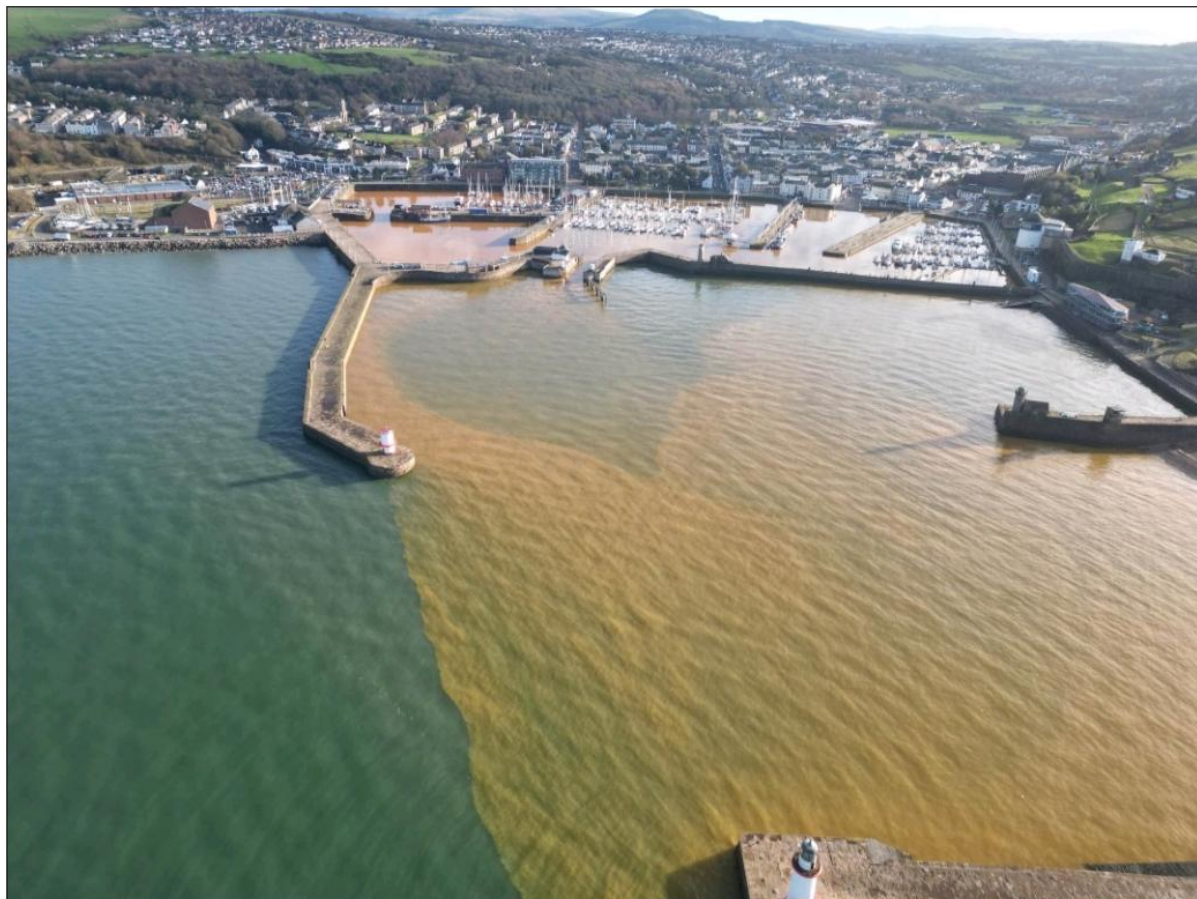
Plate 2: Photographs showing iron ochre extending into the Outer Harbour at high tide, although this was not evidenced during the site visit, it is clear that the contamination extends to the outer harbour under certain conditions.
