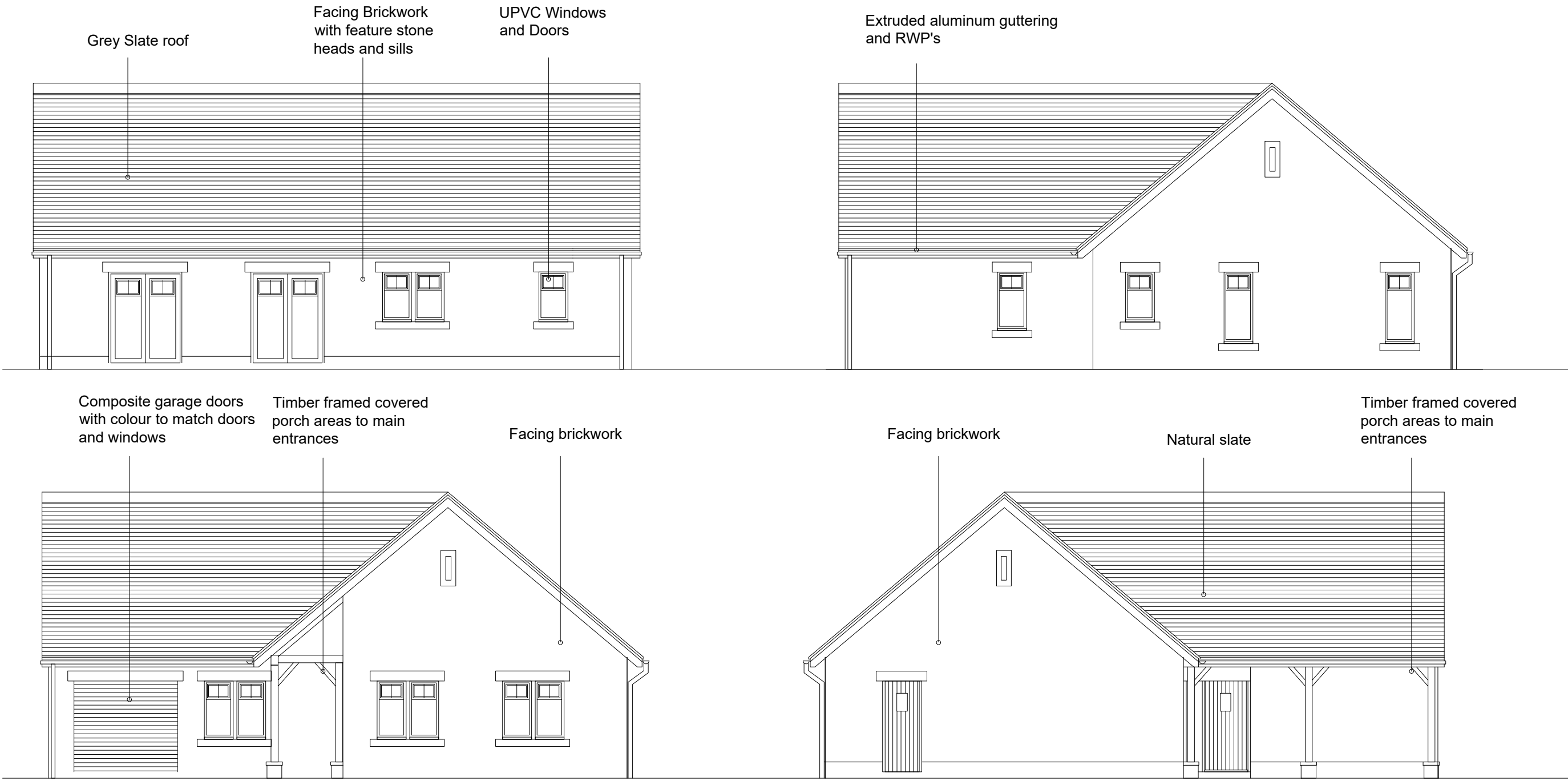
Elevations Type B 1:100
