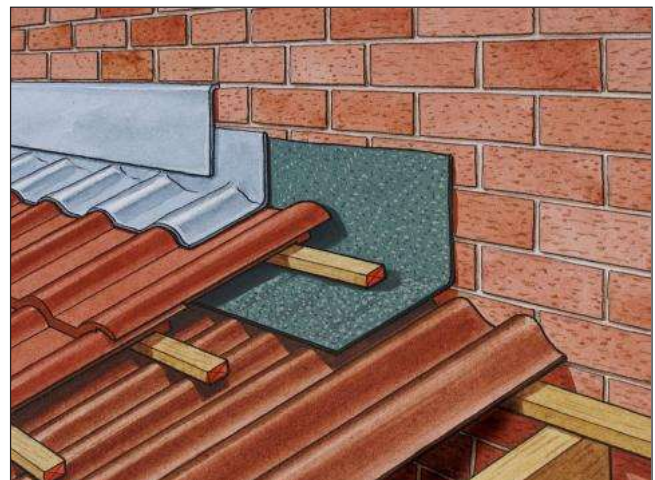
End wall abutment
