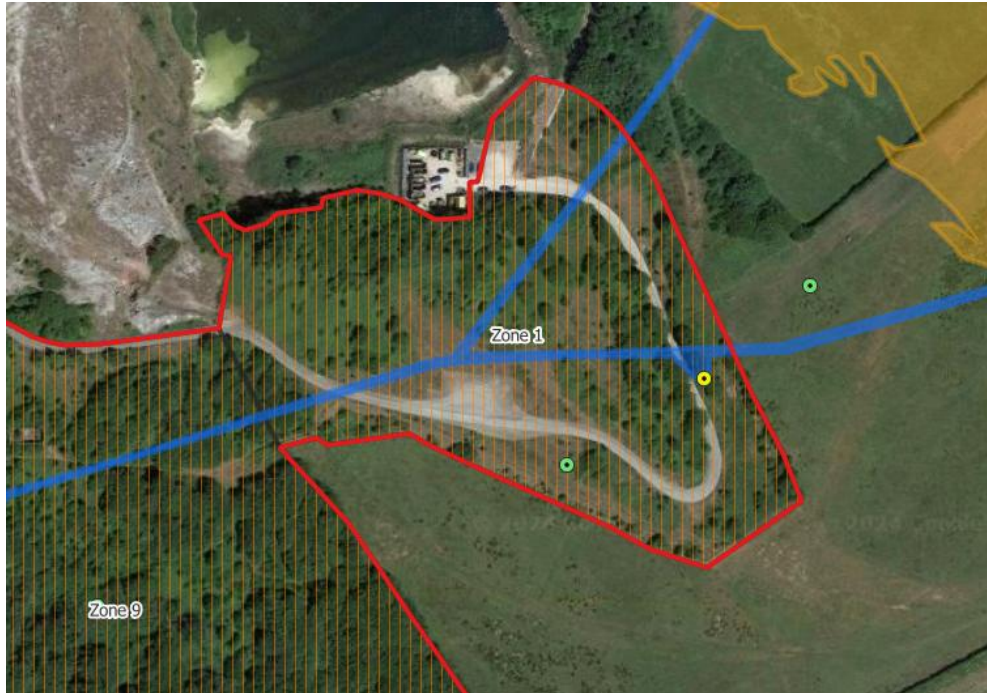
Figure 7 – Underground Mining Constraints – Development Zone 1 Site outlined in Red with Zone in Orange Hatching; Shafts/boreholes noted with green and yellow dots; Ore body workings noted by orange shading; underground road networks noted by blue shading (locations of features identified using Archive plan BDB 21-5-5-123 [Plan of Workings of Moorbank and Hodbarrow Mines. Sheet 2 Hodbarrow Mine, Owned by the Millom Heamatite Ore and Iron Co., Ltd])
