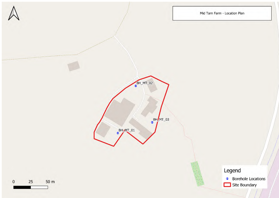
Figure 2 – Red Line Boundary and Indicative Borehole Locations
