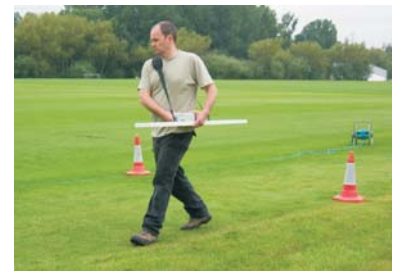
GEM-2 Multi-frequency Exploration depth up to 10m
