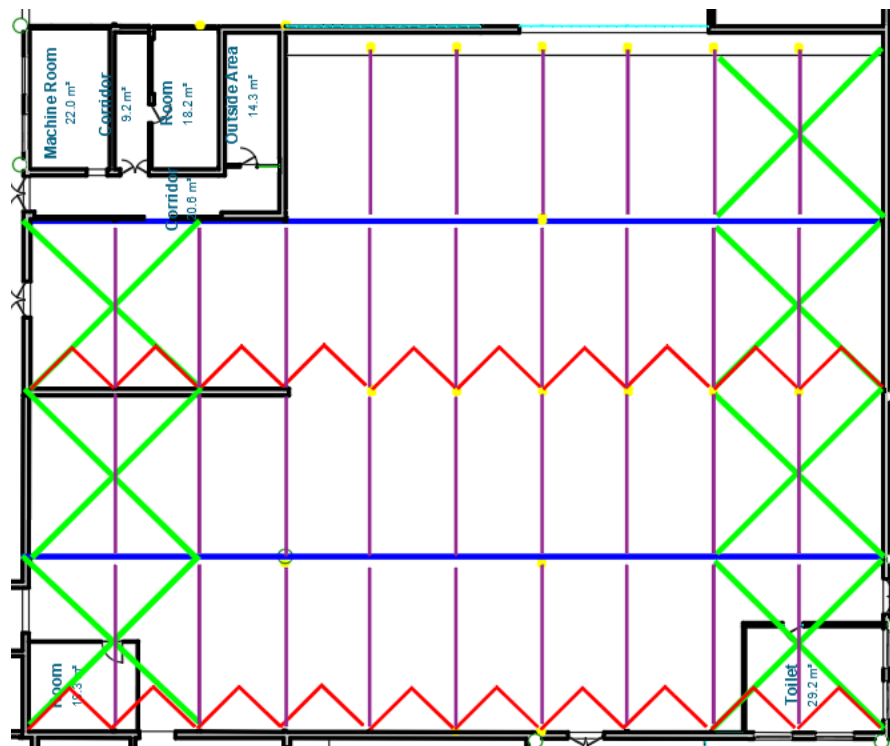
Figure 2.5 – Zone 'B' Roof Stability Systems
