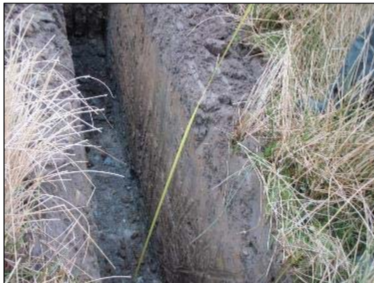
Photo 5: TP1, compact disturbed subsoil over very compact grey shale overburden.
