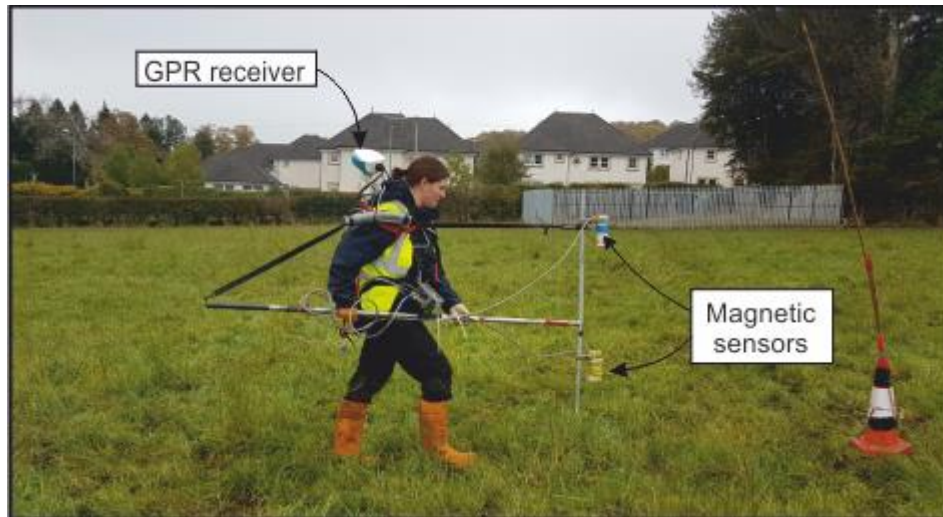
Plate 5 – G858 magnetometer (library photo).
