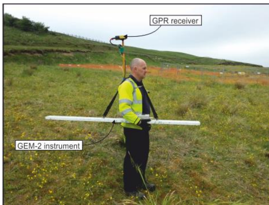
Plate 6 - GEM-2 (electromagnetic) ground conductivity meter
