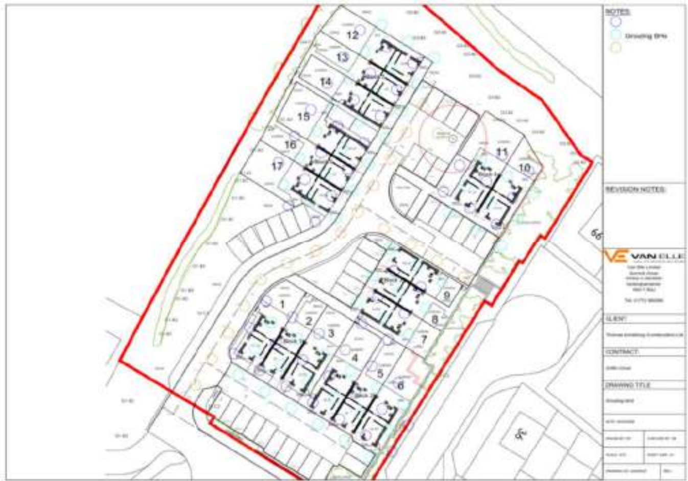
Figure 1: Drill and Grouting Borehole Plan
