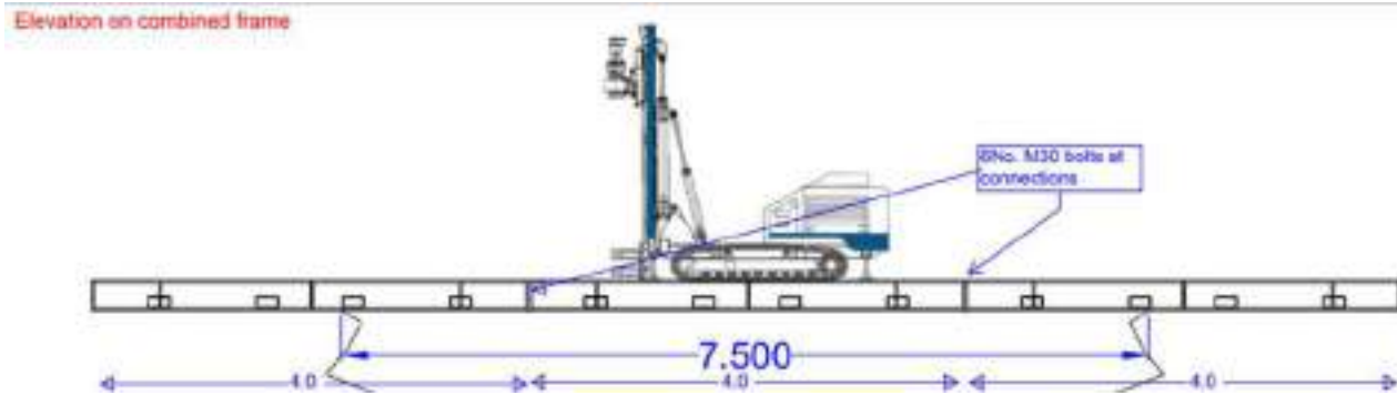
Figure 9: Example of Drill Rig on Shaft Safety Frame
