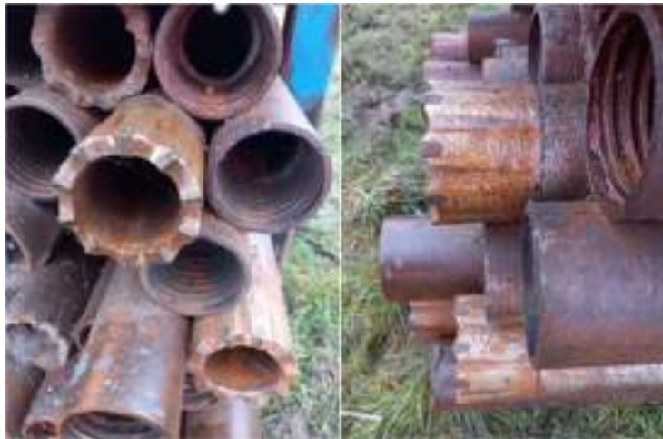
Figure 6: 101mm steel casing with cutting shoe
