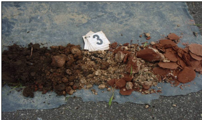
Photo 4: WS3 core failing on sandstone (right)
