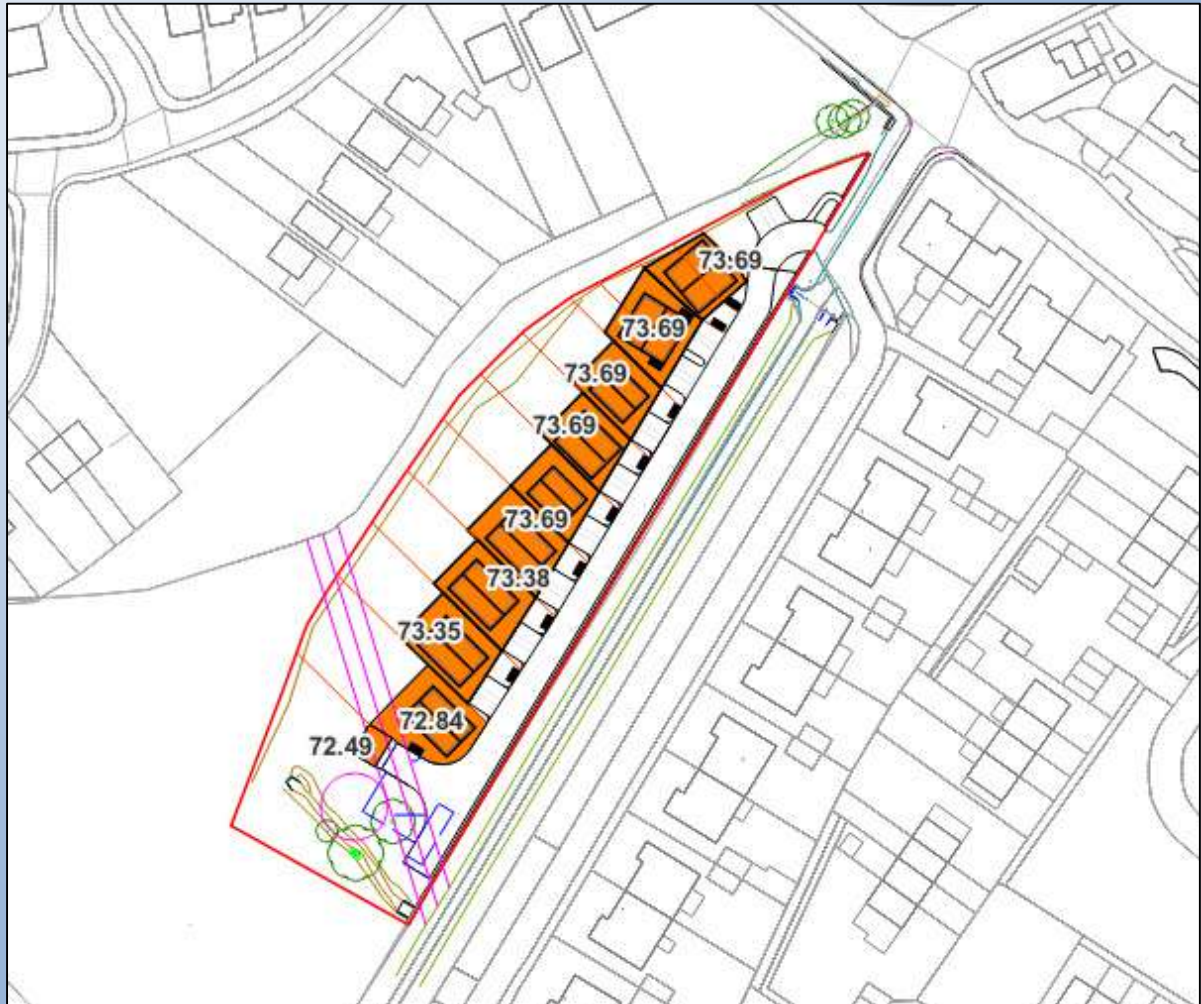
Figure 4: Proposed development finished floor levels
