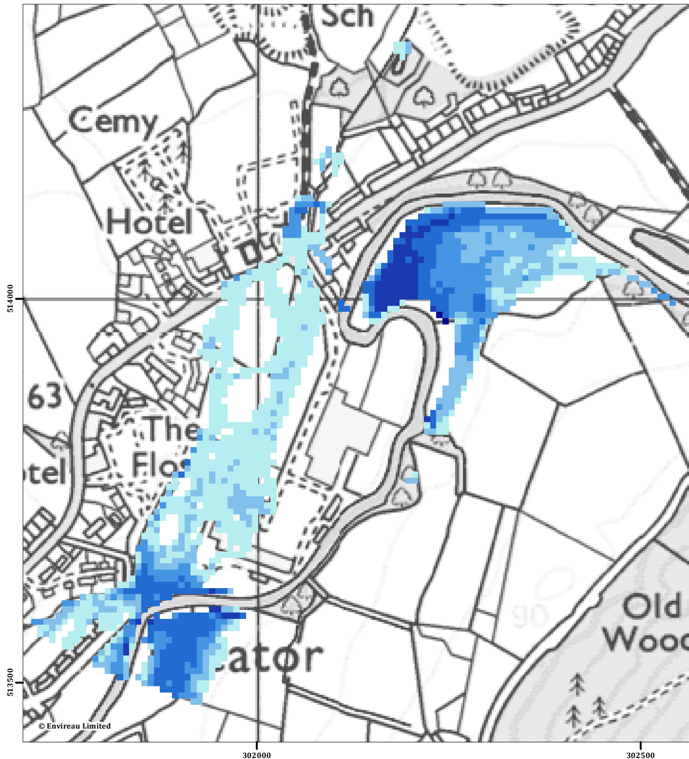
Figure 3: Tributary Flood Risk 100 year Cleator Mills
