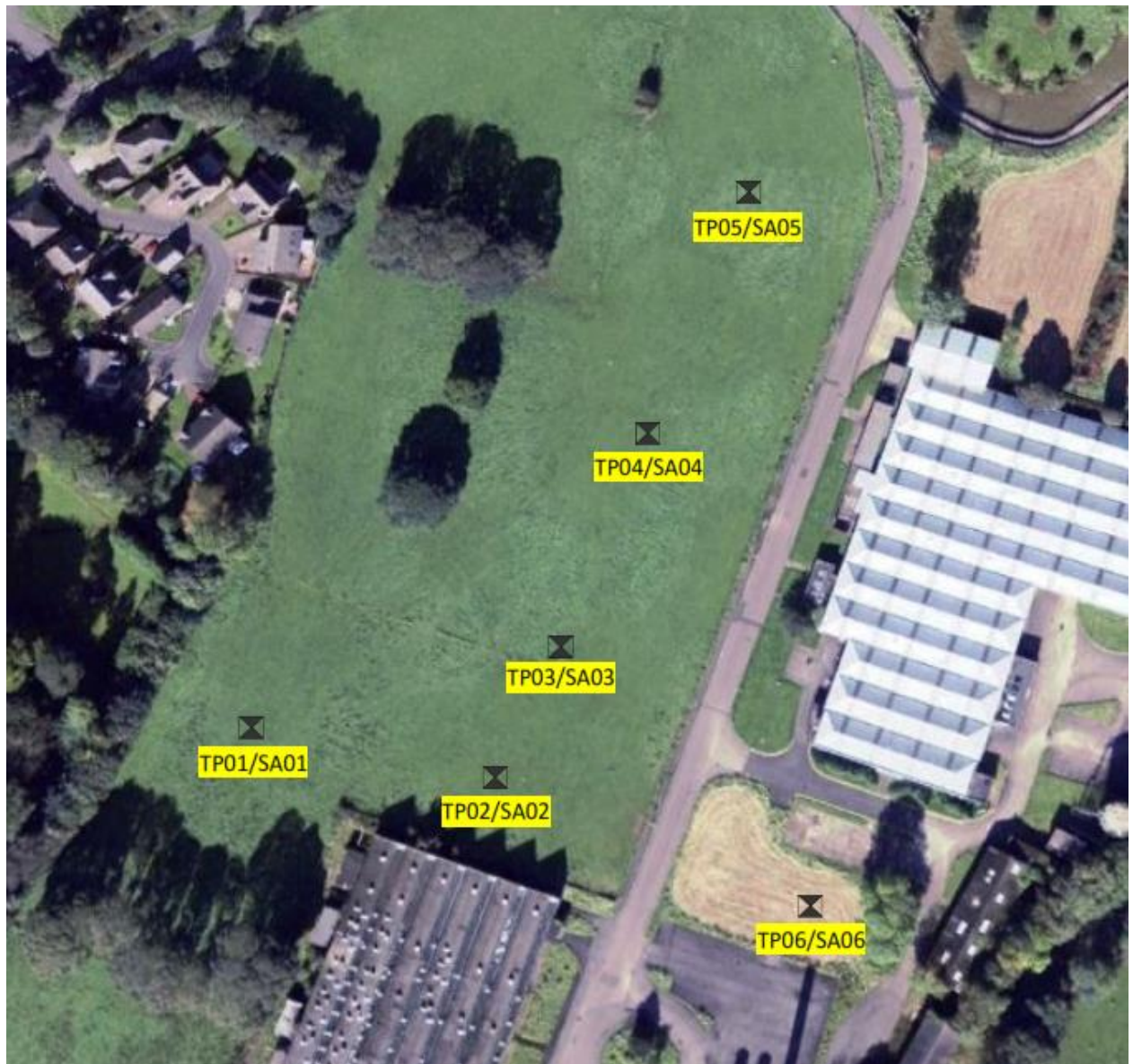
Figure 2 – Soil Infiltration Test Locations
