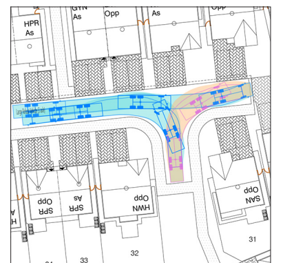
Reduced extract from i-Transport's 'Swept Path Analysis - Refuse Collection Vehicle' drawing looking at refuse access across earlier site proposals
