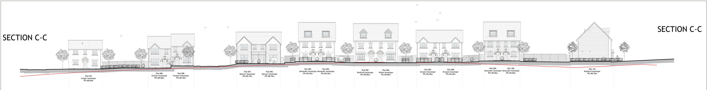
Reduced extract from drawing 64D-STO-107 - schematic streetscene / Section C-C looking at the townhouse typologies overlooking the Main Street Green Character area. Avenue street trees and estate rail fencing will be key elements in the streetscene
