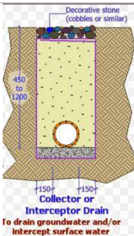
Figure 5 – Typical detail for a Granular Drain
