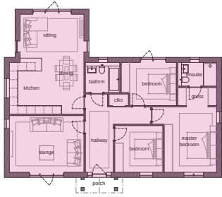
Type C Ground Floor Plan
