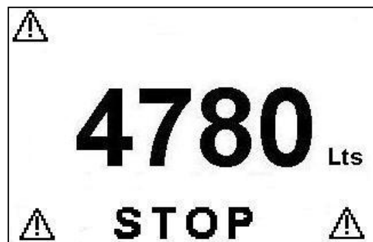
Figure 5 LCD – Overfill Alarm
